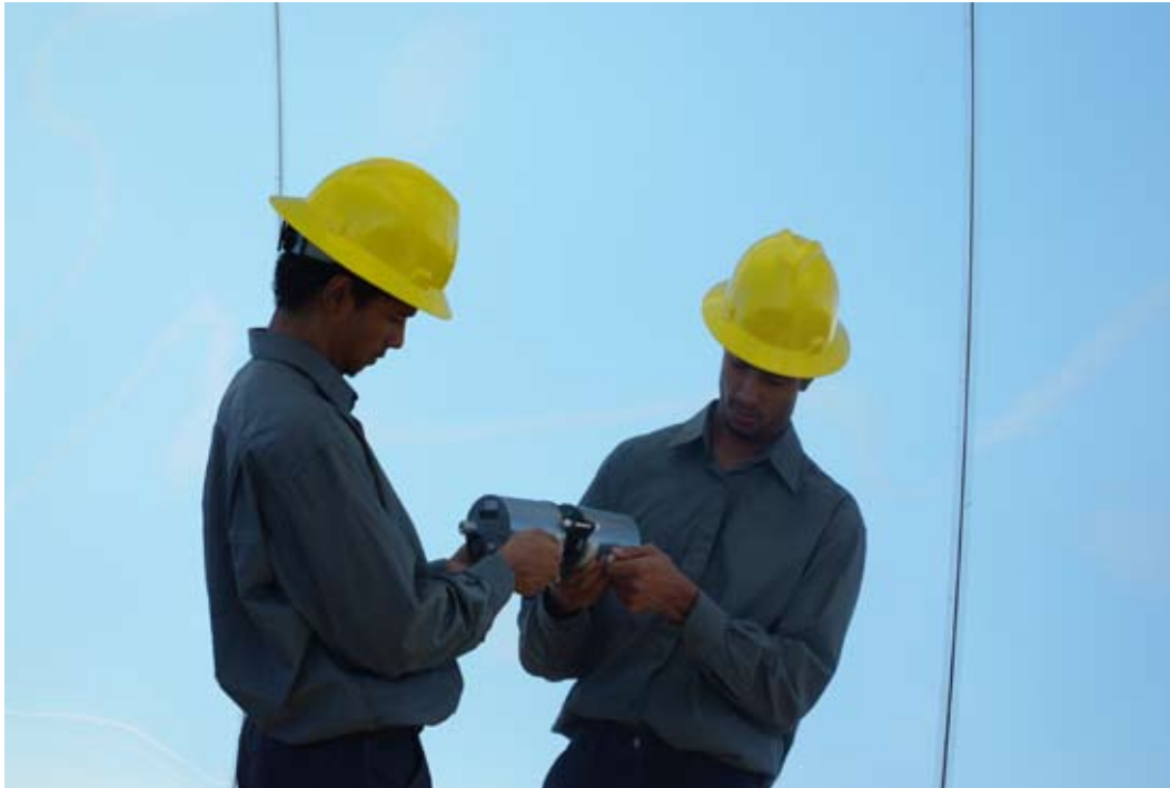
Measuring the specular reflectance of ReflecTech film on a parabolic trough concentrating solar collector.
