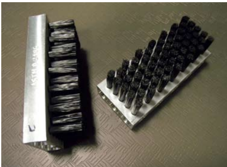
Brushes used in scrub test to simulate aggressive cleaning of ReflecTech®PLUS.
