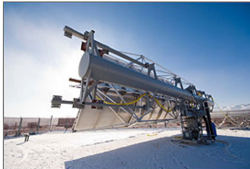
A rear view of the SkyTrough being tested atop South Table Mountain in Golden. The model is attached to NREL's Large Payload Solar Tracker. It supports solar components that require 2-axis tracking of the sun. The tracker can support equipment weighing 9,000 pounds with a tracking accuracy of 1 milliradian. Credit: Pat Corkery
