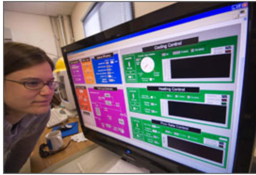
Kathleen Stynes peers at the continuous data provided by analytical instrumentation for field testing of the SkyTrough parabolic trough design. The novel design using a reflective metal coating instead of heavy glass mirrors was developed by SkyFuel with NREL's help. Credit: Pat Corkery
