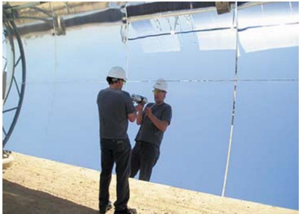
▲ ReflecTech Mirror Film co-inventor (and SkyFuel CTO) Randy Gee, measuring the reflectance of ReflecTech mirror Film panels at the SEGS VI plant in Kramer Junction, California.
