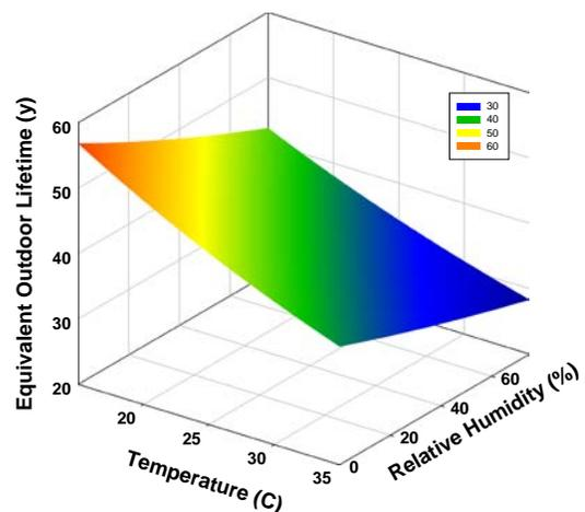
Fig. 11. Outdoor lifetime vs. temperature and relative humidity, based on  $300 \text{ MJ/m}^2/\text{y}$  UV irradiance.
