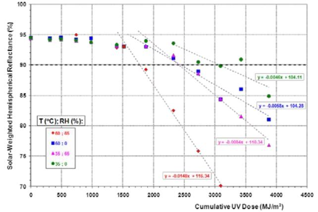
Fig. 3: Solar Simulator exposure of RT-2 samples with varying temperature and relative humidity.
