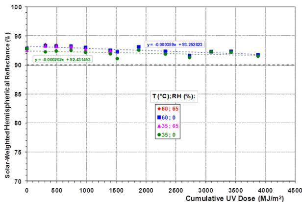
Fig. 9: Solar Simulator exposure of RT-5 samples with varying temperature and relative humidity conditions. SWHR has not yet dropped below 90%.
