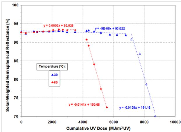
Fig. 7: UAWS exposure of RT-3 samples at 30 and 60°C. Slope of degraded part of curve is used to determine cumulative dose at which  $\rho_{2\pi}=90$ .
