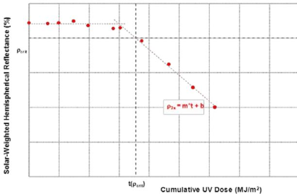
Fig. 1: Typical response of a generic metalized polymer reflector to UV exposure.
