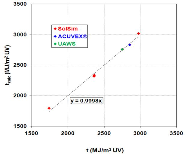
Fig. 6: Actual vs. calculated cumulative dose at  $\rho_{2\pi} = 90\%$  for RT-2 RTMF
