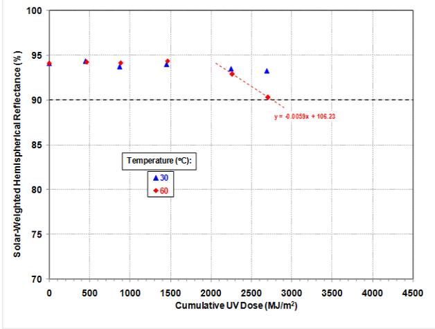
Fig. 5: UAWS exposure of RT-2 samples at 30 and 60°C.
