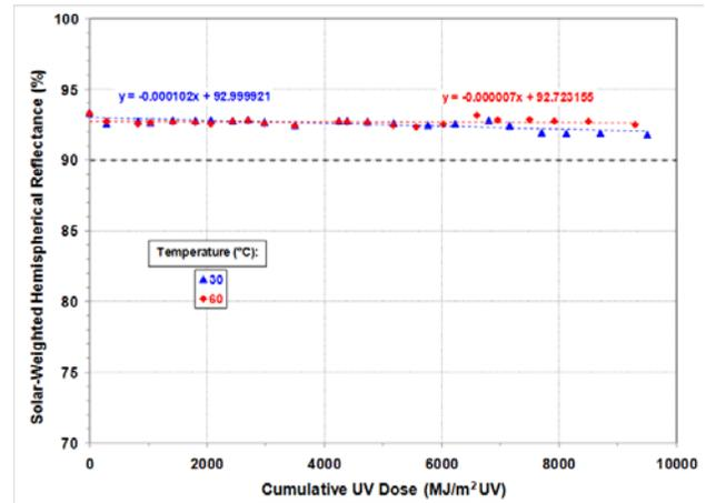
Fig. 8: UAWS exposure of RT-4 samples at 30 and 60°C. Neither SWHR data set dropped below 90%.
