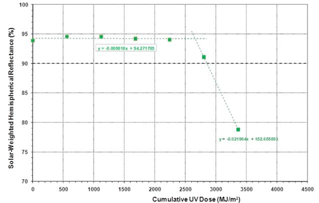
Fig. 4: ACUVEX<sup>®</sup> exposure of RT-2 samples under time varying environmental conditions.
