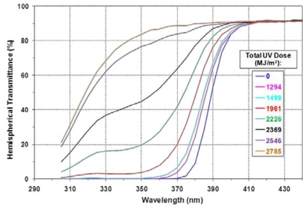
Fig. 2: Spectral transmittance of prototype UV screening film as a function of total UV dose (Ci5000).
