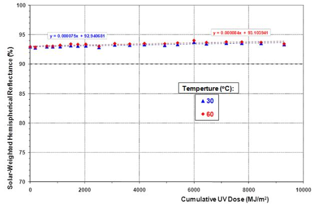
Fig. 10: UAWS exposure of RT-5 samples at 30 and  $60^\circ\text{C}$ . The SWHR of neither data set has dropped below 90%.
